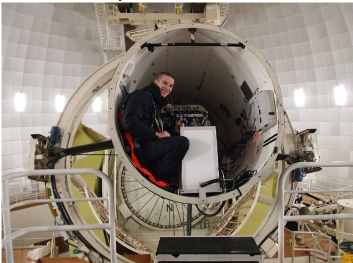
Figure 1: SAMI team member Sam Richards prepares for a long winter's night riding in the prime focus cage of the AAT monitoring the instrument alignment and plugging hexabundles into the pre-drilled plates. (Image credit: AAO, U. Sydney)
