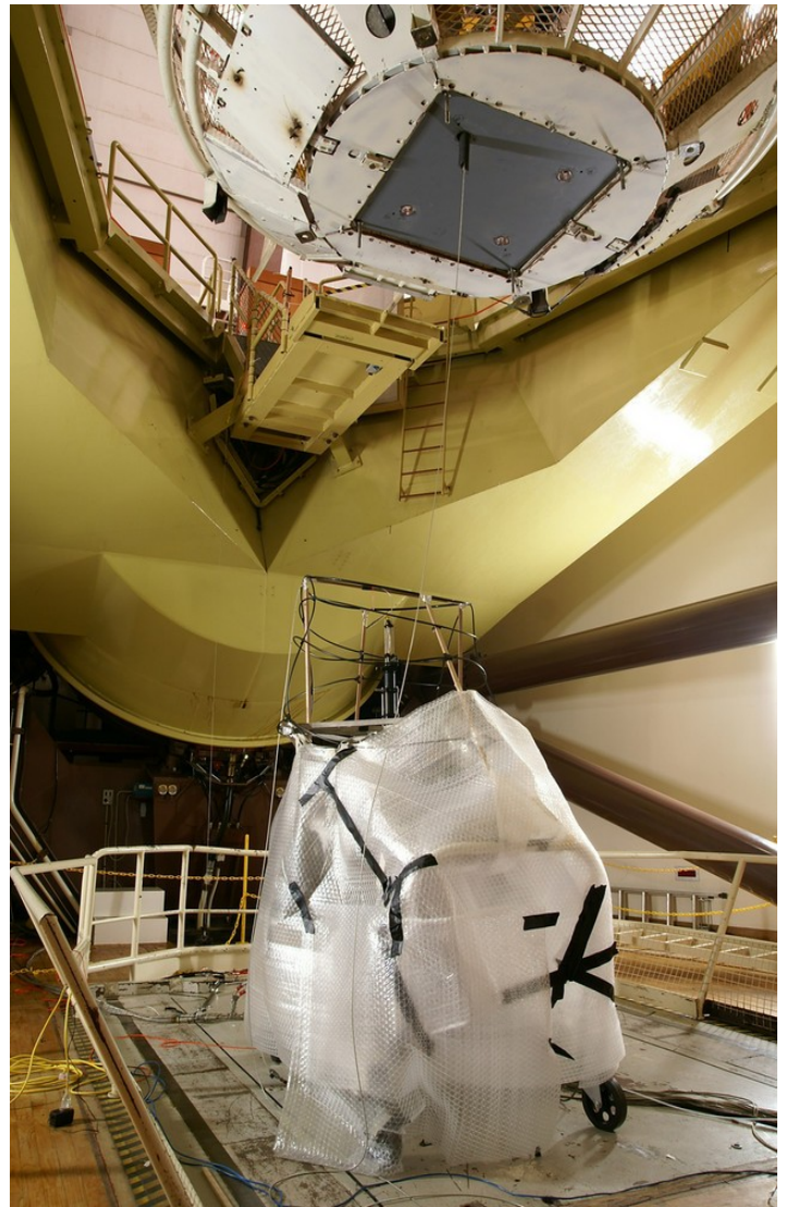
The GNOSIS optical fibre runs from the Cassegrain feed of the AAT at top, down to the IRIS2 instrument below which is wrapped Christo-like in bubble-wrap to prevent the delicate optical fibre from snagging on IRIS2 as the telescope tracks the target of interest (Image credit: Anthony Horton, AAO)
