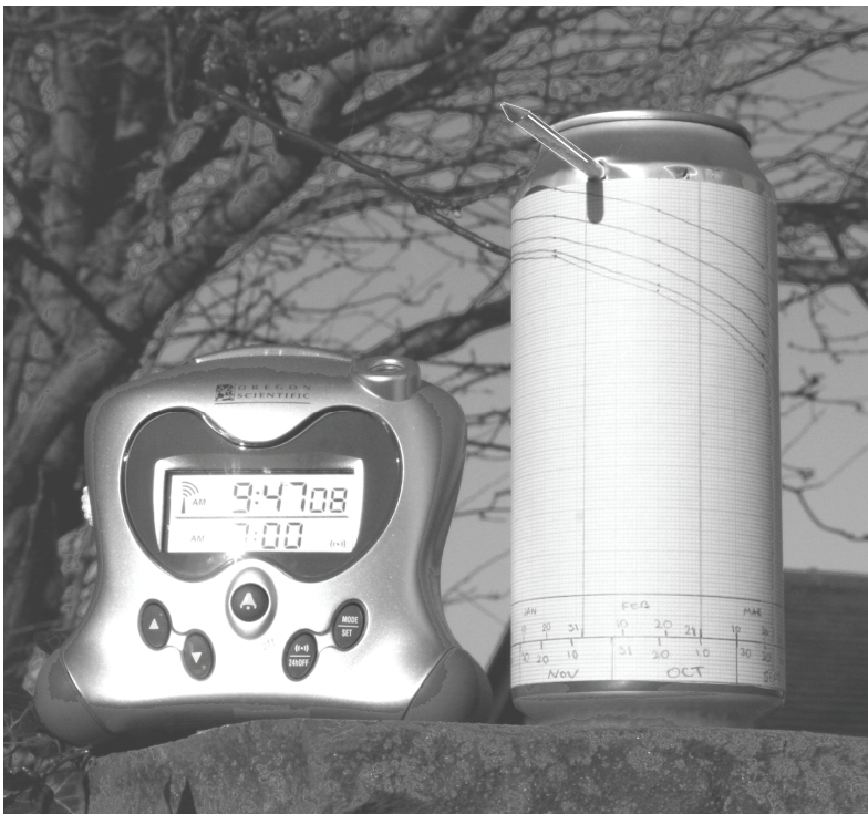
Coke-can sundial. Photo courtesy of Lydia Rex
