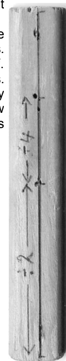
(Right) The cross arm, roughly full size, showing the positions to insert the four pins, and the scale factors for each. Note the centre line, which should also be drawn on the underside of the cross arm
