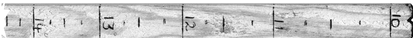
(Above, top) the "eye -end" of the staff, showing scale details, reproduced roughly full-size. (Below) The "sky end" of the scale (also shown full size) is distinguished by the little notch in the end. This is the end featured in the photograph (top left)
