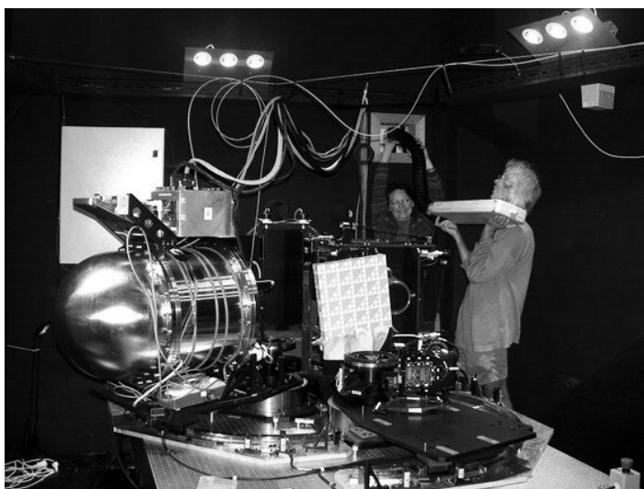
The head of the snake arrives inside the AAOmega spectrograph room, where it is “wrestled” by Instrument Scientist Will Saunders. The large bulbous cylinder on the left houses the “blue” camera. (Images courtesy Steve Lee, AAO)
