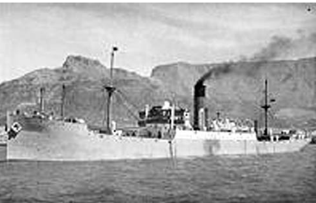
Sandown Castle was built in 1921 by Short Bros. in Sunderland with a tonnage of 7607grt. She was built as a cargo only ship and operated between the USA and South Africa, occasionally sailing to the UK. She was scrapped in 1950. (Photo: A Duncan)
