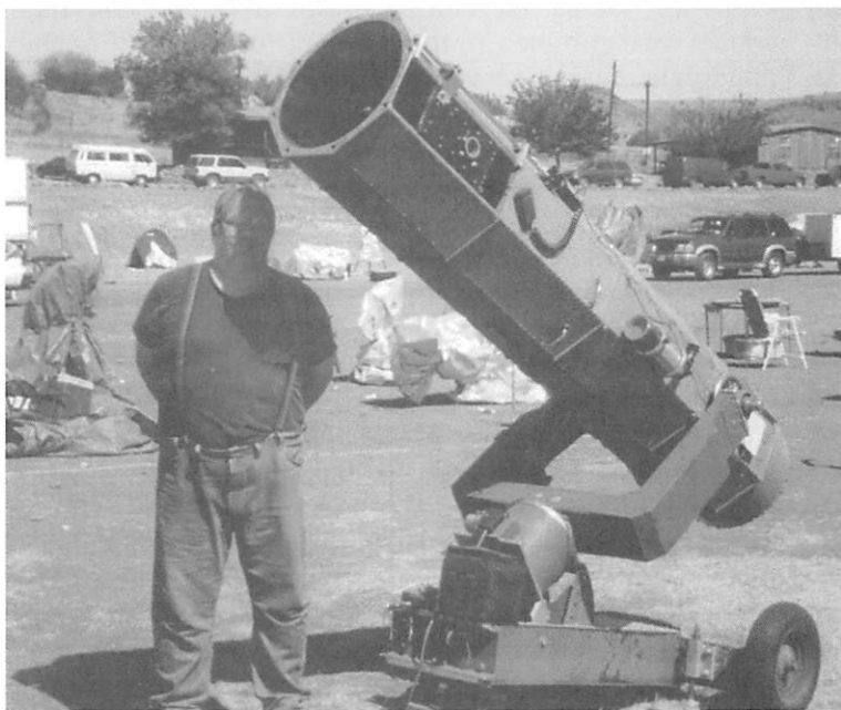
Gil Machin, of Kansas City Missouri, with his homemade 400mm Newtonian telescope, for which he made his own mirror, clearly showing the equatorial drive and the facility for moving and levelling the instrument Photo by Michael Bakich, the author of this new book.
