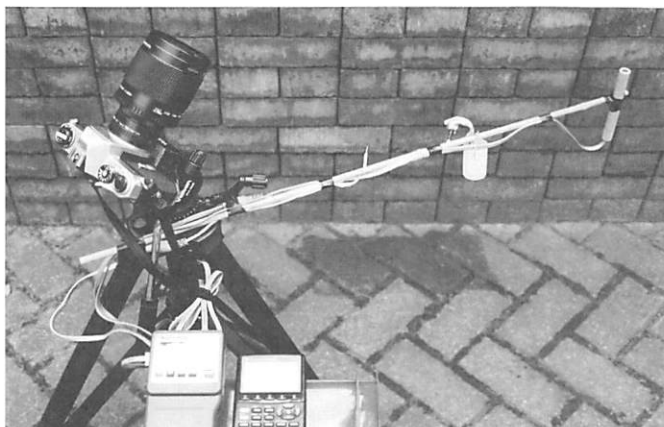
Alan Pickwick's SLR camera as set up to take the photograph on page 1, together with the light and temperature measuring equipment.
