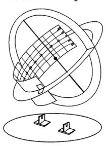
shown. The two intersecting joins should be filleted with a solid-setting resin glue. Make a gnomon of length 2R from a straight piece of thick wire (from a dry-cleaner's coat hanger) and fix a bead in the centre. Then glue the gnomon diametrically across the meridian ring at 90 degrees from the join with the equatorial ring.
