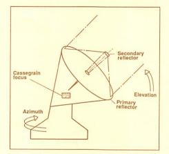
and azimuth are made using direct current torque motors acting through frictional contact.
